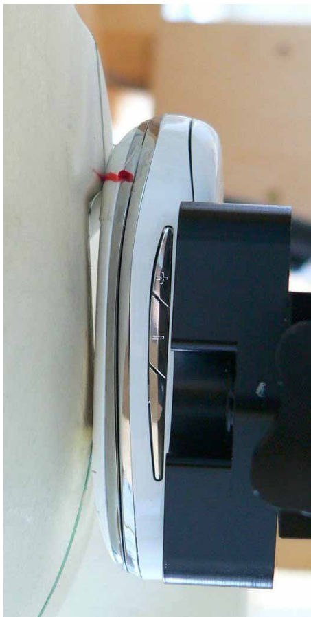
Fig. 27: Cheek position, left side, slider down.
