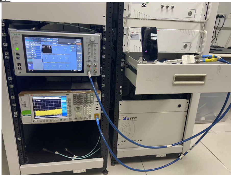
RF Conducted Test setup (GSM/WCDMA/LTE)
