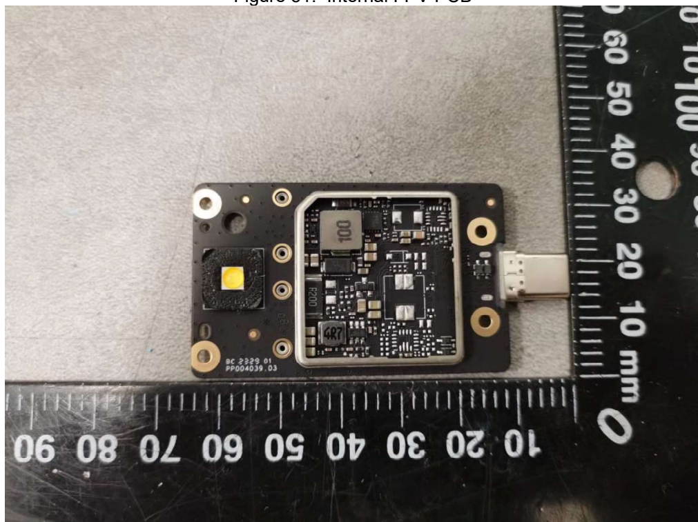
Figure 52. Internal FPV PCB (metal shield removed)
