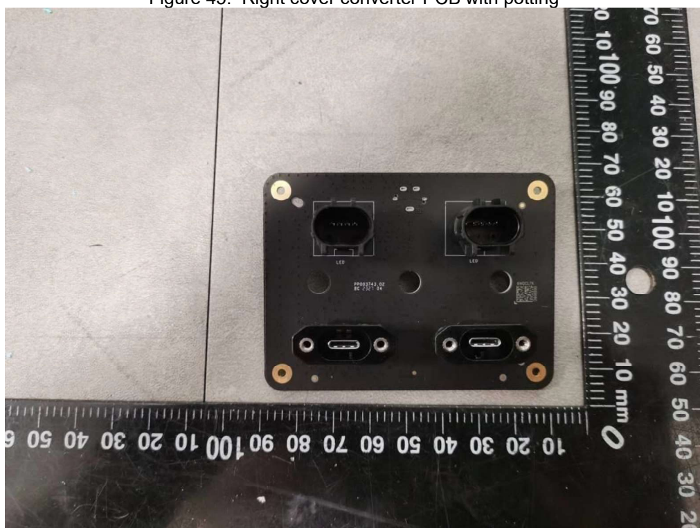
Figure 46. Right cover converter PCB with potting removed
