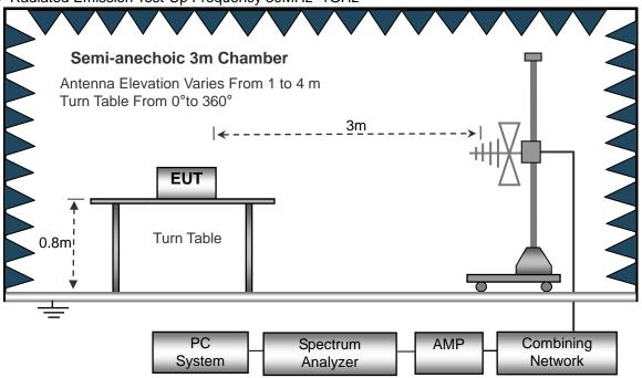
(C) Radiated Emission Test-Up Frequency Above 1GHz
