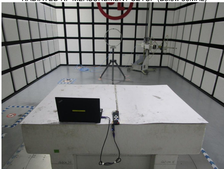
RADIATED RF MEASUREMENT SETUP (Below 30MHz)
