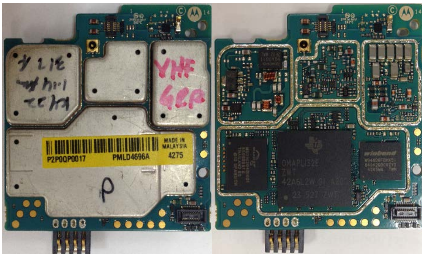
RF board with and without Shields (Bottom)
