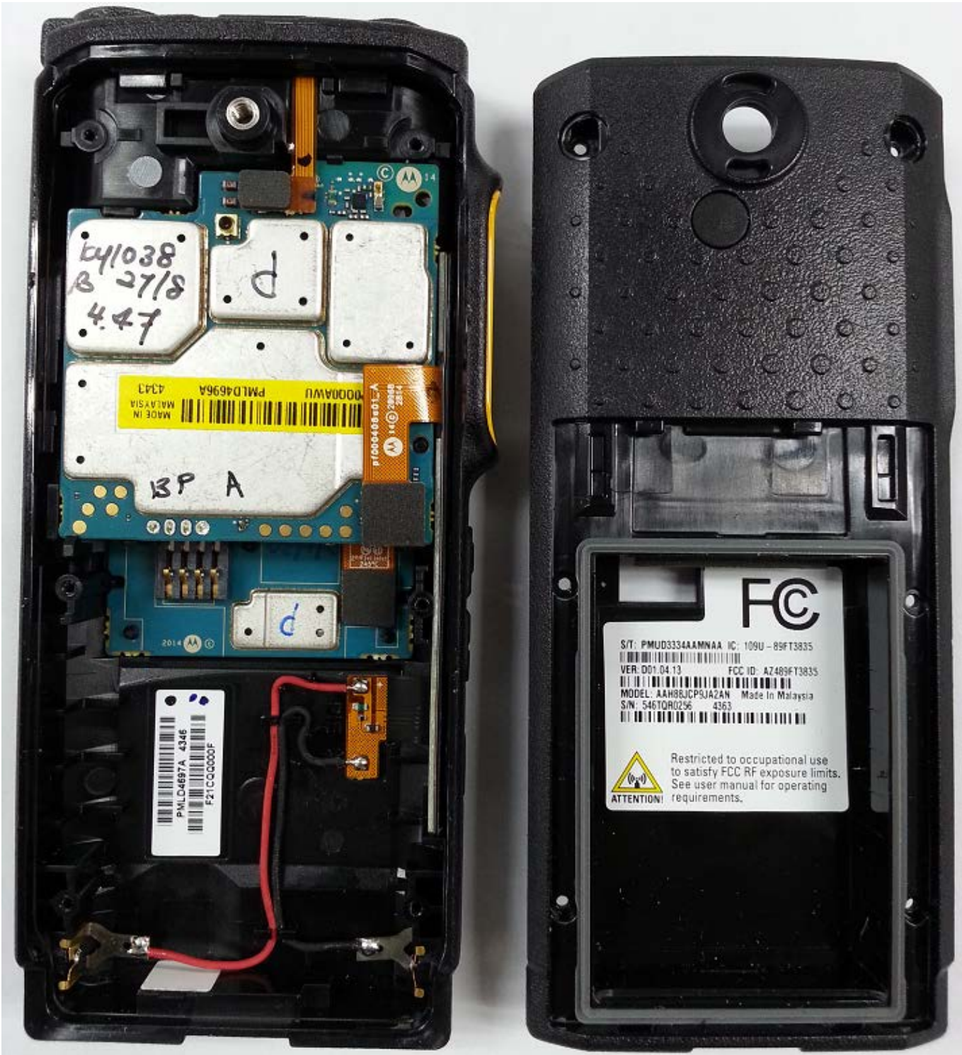
PCB board with chassis and housing for Display Model (Bottom)
