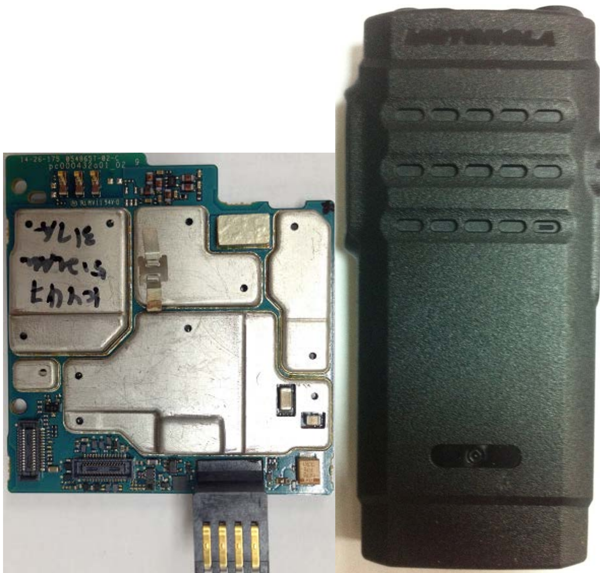
PCB board with chassis and housing (Top)
