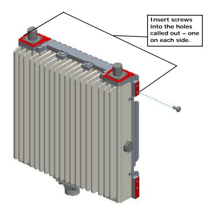
Hang the RP to the mounting bracket using the installed screws. Align holes at bottom location of bracket and install two additional screws. Tighten all four screws.
