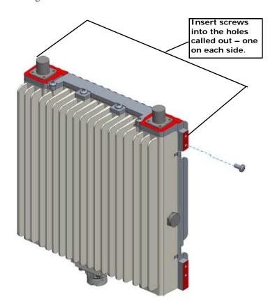
Attach the RP to the mounting plate. Tighten the screws on the RP.
