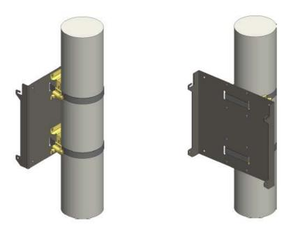
Insert two screws into the upper holes on opposite sides of the RP as shown in the drawing below.
