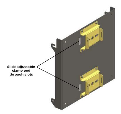
**2** Wrap each clamp around the pole and tighten the clamp screw to secure the RP to the pole.
