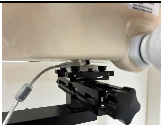
Horizontal-Down of EUT with 0 cm Gap
