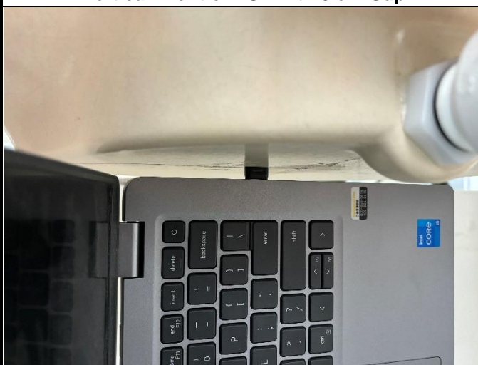
Tip Mode of EUT with 0 cm Gap
