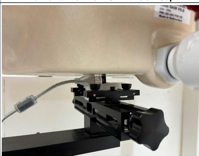
Vertical-Back of EUT with 0 cm Gap
