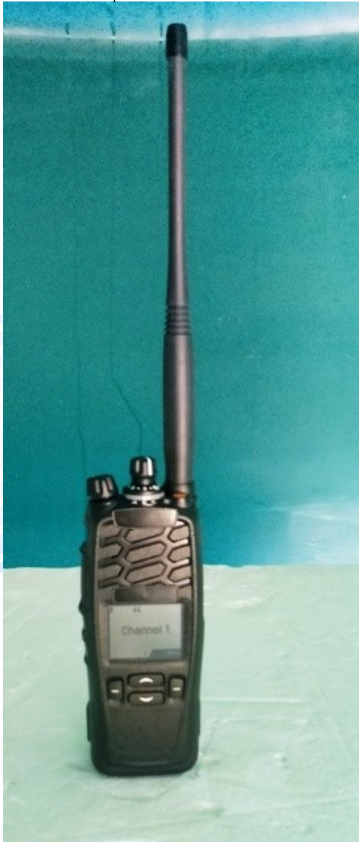
Test sample with VHF antenna attached
