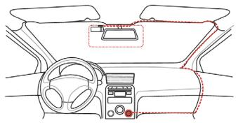
Onnect the USB cable with camera and Car adapter. When the car starts up, the camera will boot up automati cally with voice prompt "Hello".
