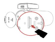
1 Insert the TF Card into the Slot (note the direction).
