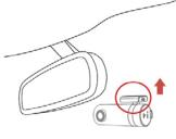
Stick the plastic stent onto the windshield ( note the position ).
