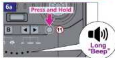
Fig. 6a Press and hold the Volume Up+ Button 11 while powering on the device. The transmitter will emit a Long Beep sound.
