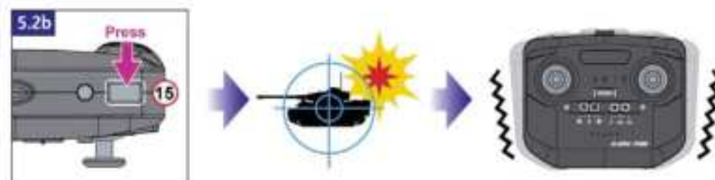
Fig. 5.2b Beside the transmitter will vibrate when the press Cannon Switch 15 is fired or hit by infrared during battle.
