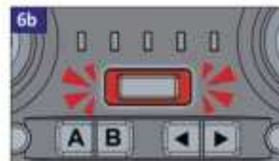
Fig. 6b The Engine LED will flash . Indicating that the joystick potentiometer center point adjustment mode has been entered.
