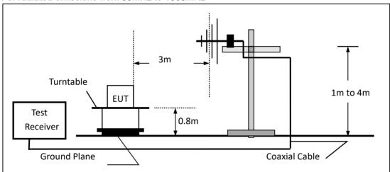
(c) For radiated emissions above 1000MHz
