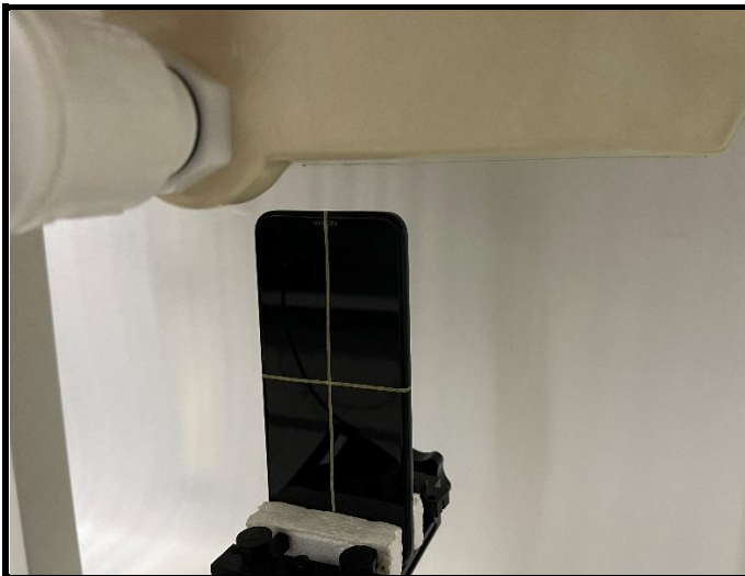
Bottom Side of EUT with 2.0 cm Gap
