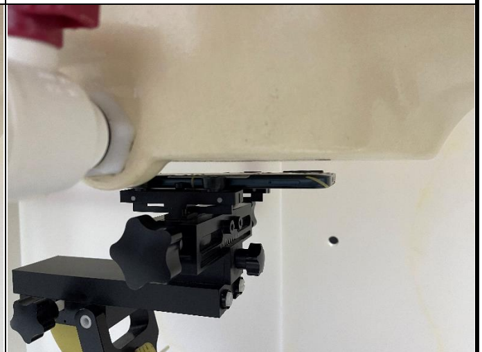
Rear Face of EUT with 1.0 cm Gap
