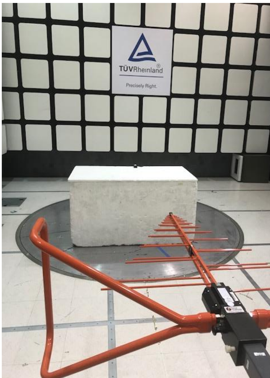
Figure 5 - Radiated Emissions Test Setup 30 - 1000 MHz – Front
