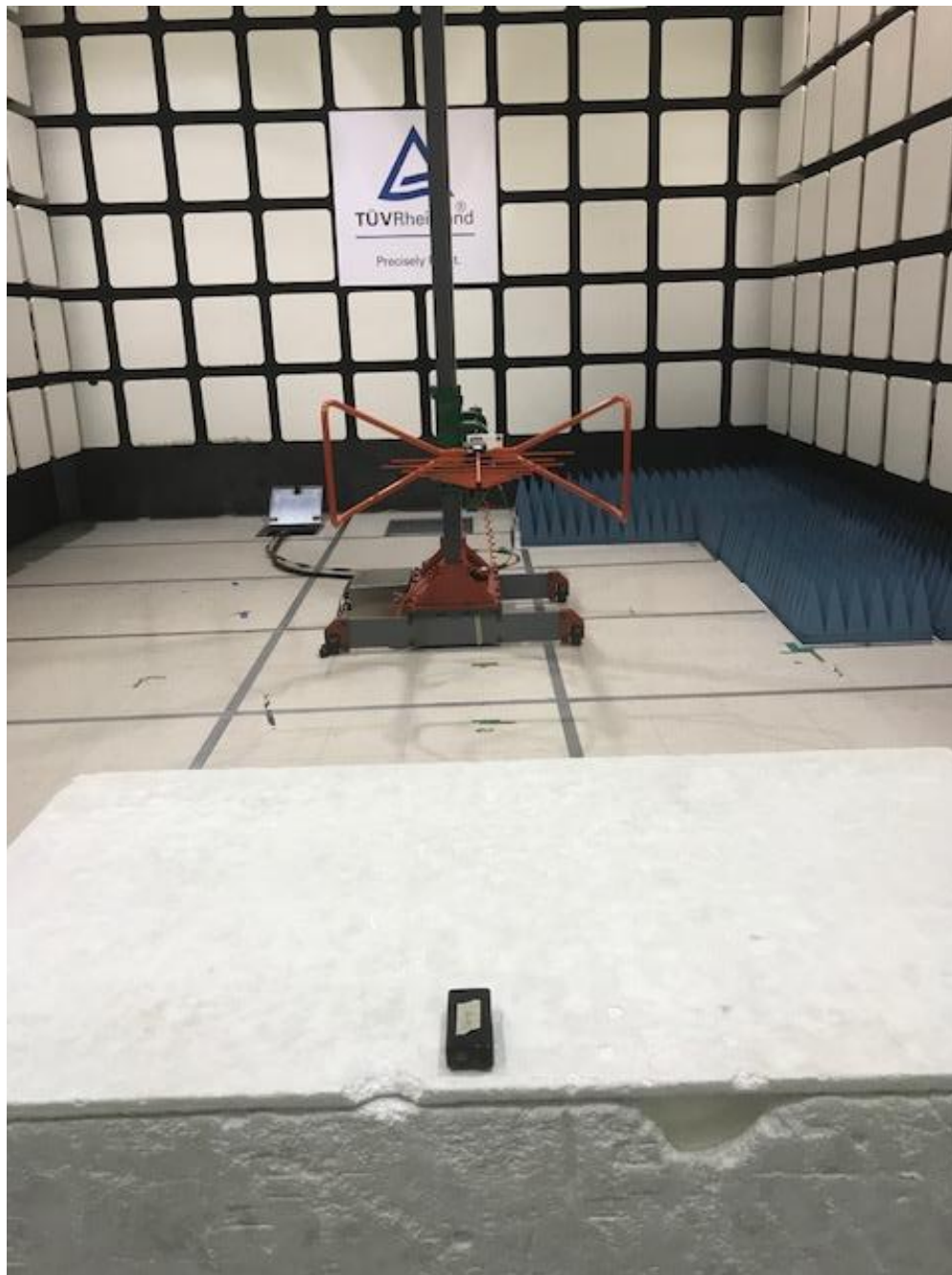
Figure 6 - Radiated Emissions Test Setup 30 - 1000 MHz – Back
