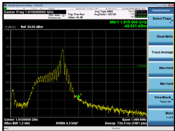
NB-IoT Band 25 QPSK 15kHz 12@0 CH-High
