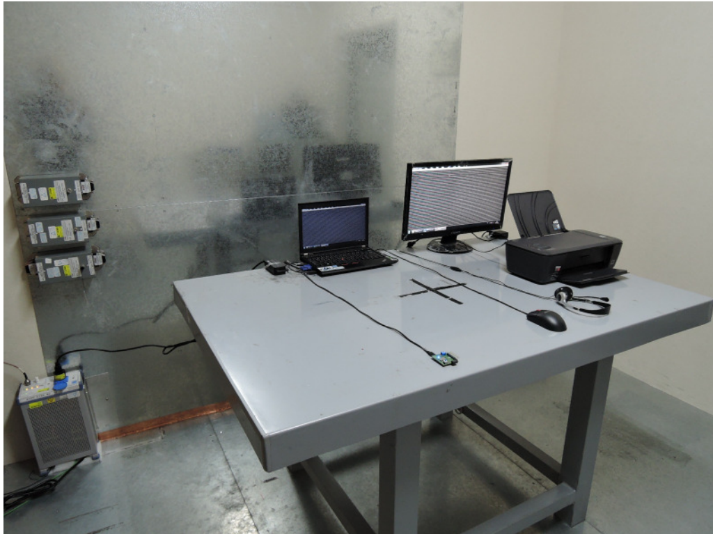
Photograph 6: Set-up for for Mains Conducted testing Front
