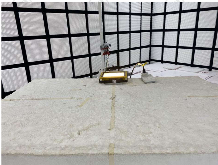
Radiated spurious emission Test Setup-2(Above 1GHz)
