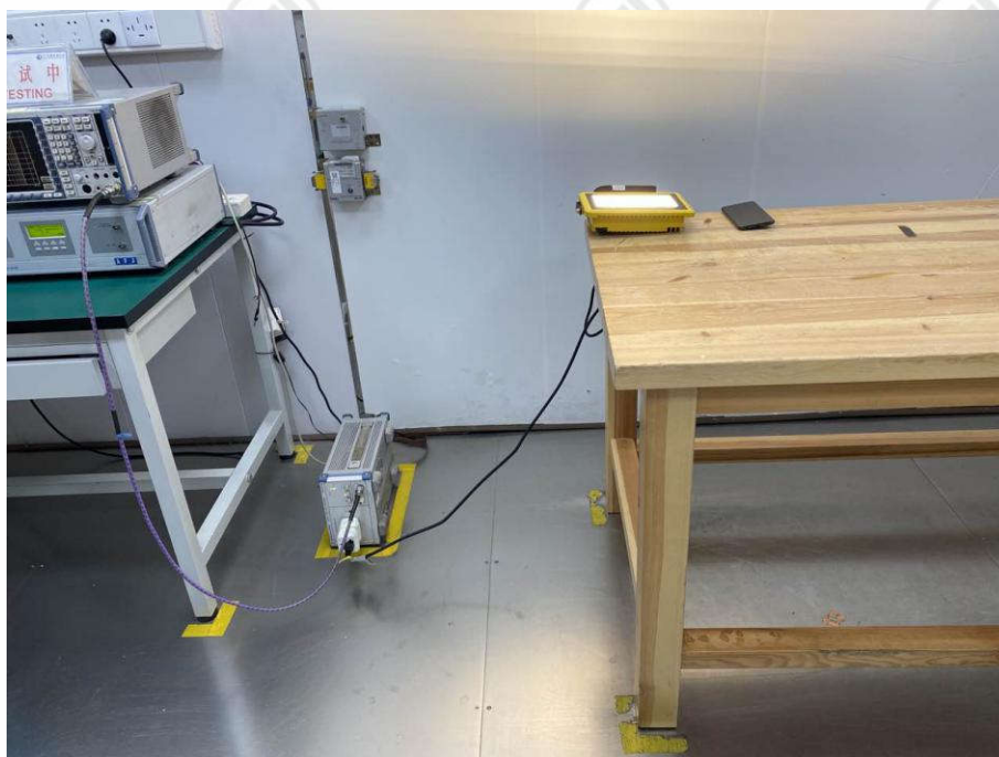
AC Power Line Conducted Emission Test Setup
