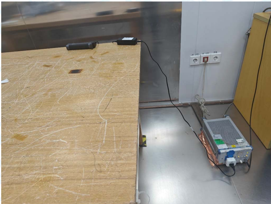
Photo of Setup for Conducted Emission
