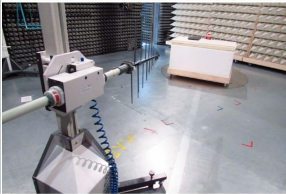
Setup for TX measurement below 1 GHz
