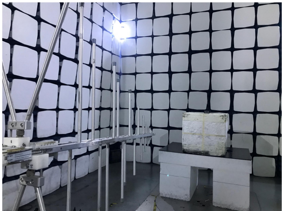
Radiation Emission Test Setup (30MHz to 1GHz)
