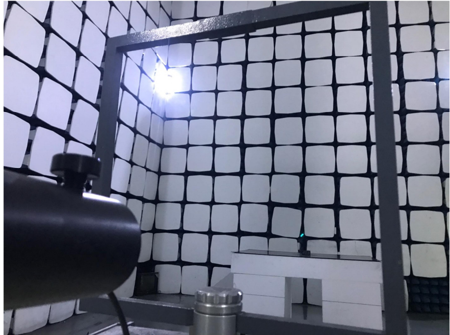
Radiation Emission Test Setup (Below 30MHz)
