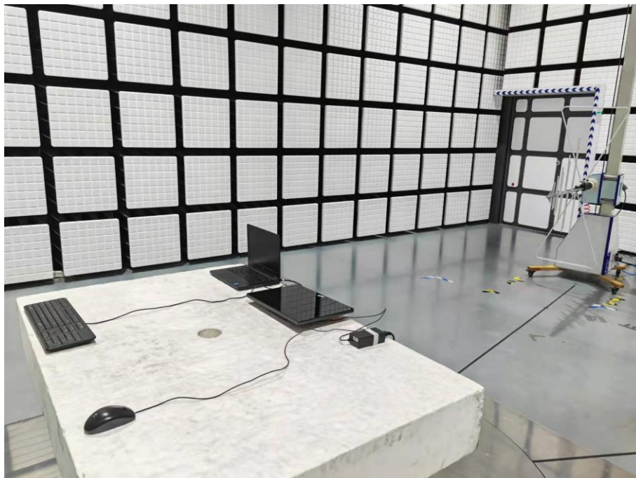
Description: Back view of Radiated Emission Test Setup
