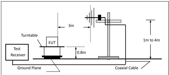
(c) For radiated emissions above 1000MHz
