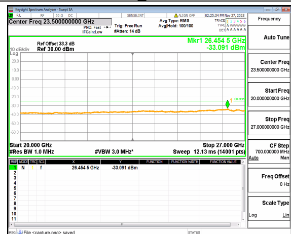
n41 (20GHz-27GHz) 50M DFT-s-OFDM QPSK Edge_1RB_Left Mid
