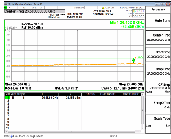
n41 (20GHz-27GHz) 60M DFT-s-OFDM QPSK Outer_Full Mid
