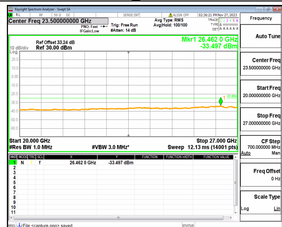
n41 (20GHz-27GHz) 60M DFT-s-OFDM BPSK Edge_1RB_Left Low
