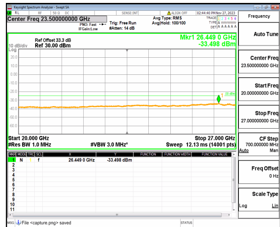
n41 (20GHz-27GHz) 60M DFT-s-OFDM BPSK Edge_1RB_Right Mid
