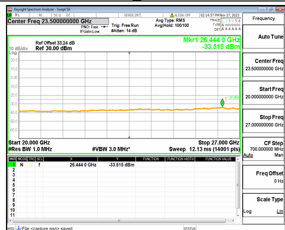
n41 (20GHz-27GHz) 50M DFT-s-OFDM BPSK Edge_1RB_Left Low
