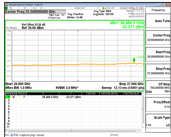
n41 (20GHz-27GHz) 70M DFT-s-OFDM QPSK Outer_Full Low
