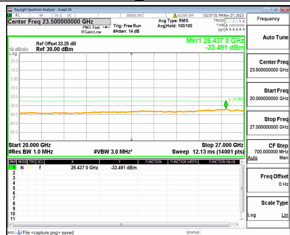
n41 (20GHz-27GHz) 70M DFT-s-OFDM BPSK Edge_1RB_Left Low
