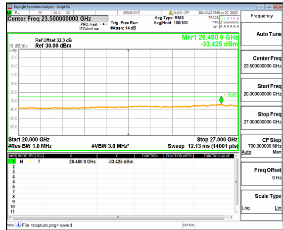
n41 (20GHz-27GHz) 60M DFT-s-OFDM BPSK Outer_Full Mid
