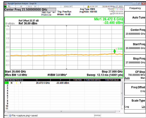
n41 (20GHz-27GHz) 40M DFT-s-OFDM BPSK Outer_Full High
