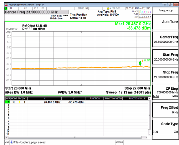
n41 (20GHz-27GHz) 60M DFT-s-OFDM QPSK Edge_1RB_Right High
