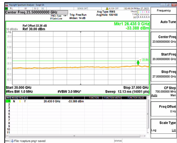
n41 (20GHz-27GHz) 60M DFT-s-OFDM BPSK Outer_Full_High
