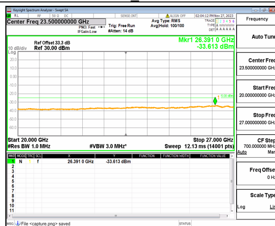
n41 (20GHz-27GHz) 40M DFT-s-OFDM QPSK Edge_1RB_Left Mid
