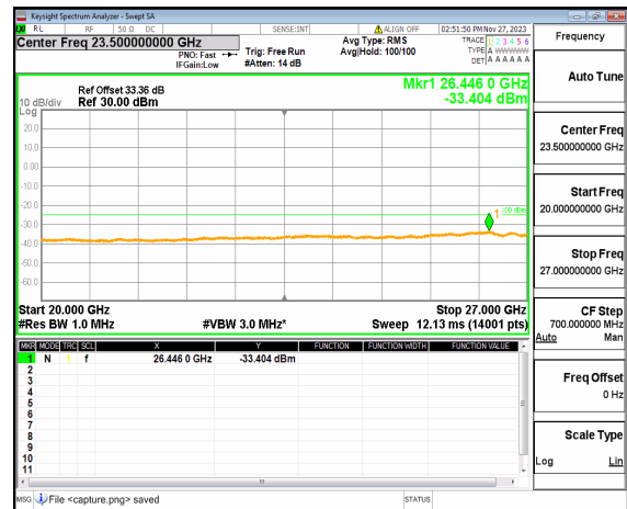
n41 (20GHz-27GHz) 60M DFT-s-OFDM BPSK Edge_1RB_Right High
