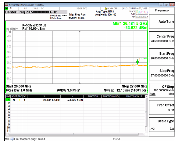
n41 (20GHz-27GHz) 50M DFT-s-OFDM QPSK Outer_Full High
