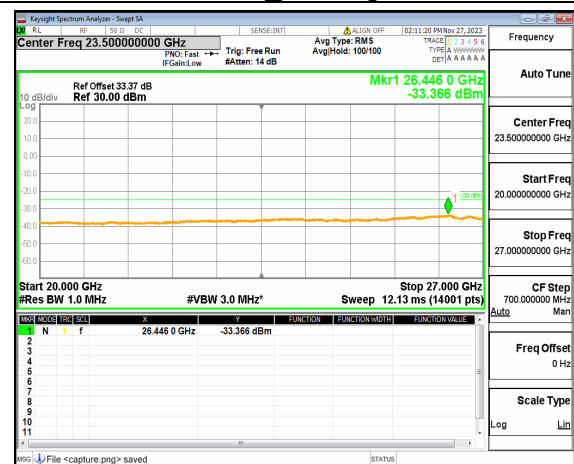
n41 (20GHz-27GHz) 40M DFT-s-OFDM QPSK Edge_1RB_Left High
