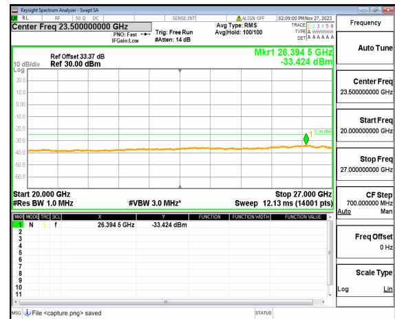
n41 (20GHz-27GHz) 40M DFT-s-OFDM BPSK Edge_1RB_Right High
