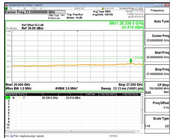
n41 (20GHz-27GHz) 60M DFT-s-OFDM QPSK Edge_1RB_Right Mid
