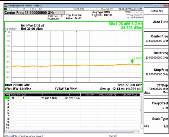
n41 (20GHz-27GHz) 60M DFT-s-OFDM QPSK Edge_1RB_Left High
