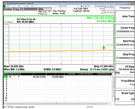
n41 (20GHz-27GHz) 60M DFT-s-OFDM QPSK Edge_1RB_Right Low
