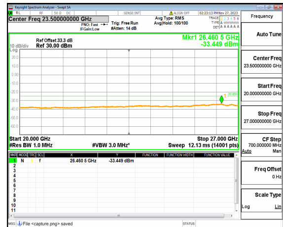
n41 (20GHz-27GHz) 50M DFT-s-OFDM BPSK Edge_1RB_Right Mid
