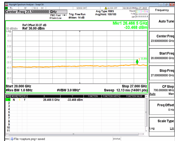
n41 (20GHz-27GHz) 50M DFT-s-OFDM BPSK Edge_1RB_Right High
