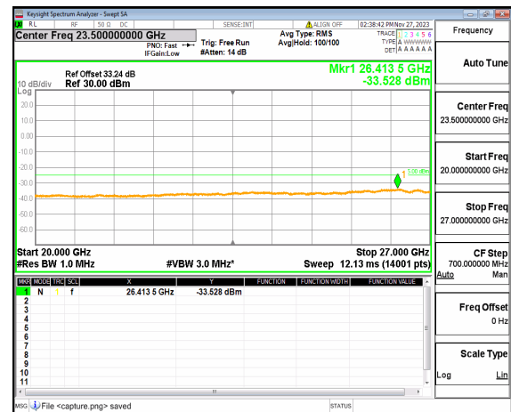
n41 (20GHz-27GHz) 60M DFT-s-OFDM QPSK Outer_Full Low
