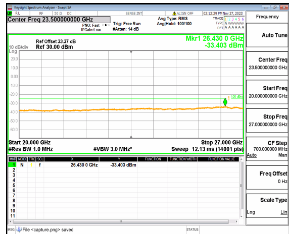
n41 (20GHz-27GHz) 40M DFT-s-OFDM QPSK Edge_1RB_Right High
