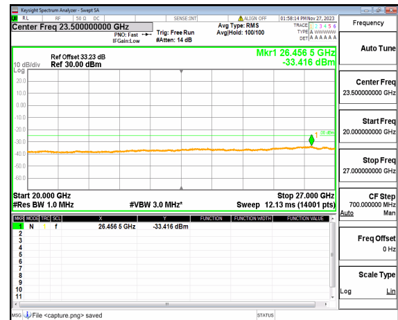
n41 (20GHz-27GHz) 40M DFT-s-OFDM QPSK Edge_1RB_Right Low
