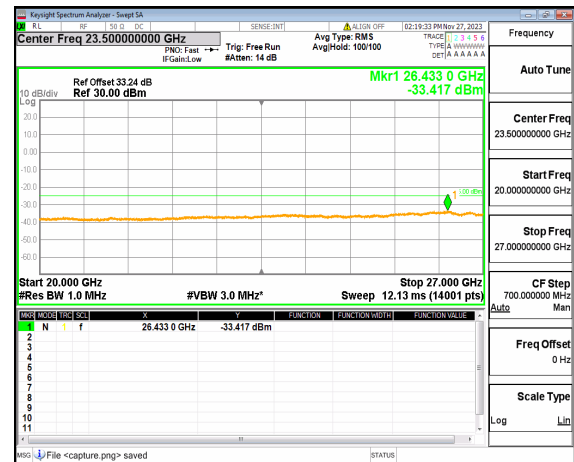
n41 (20GHz-27GHz) 50M DFT-s-OFDM QPSK Edge_1RB_Right Low
