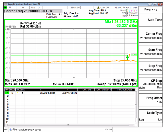
n41 (20GHz-27GHz) 50M DFT-s-OFDM QPSK Edge_1RB_Right Mid
