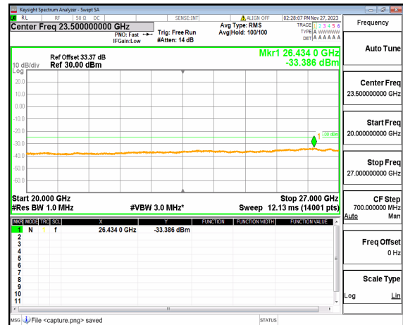
n41 (20GHz-27GHz) 50M DFT-s-OFDM BPSK Outer_Full_High
