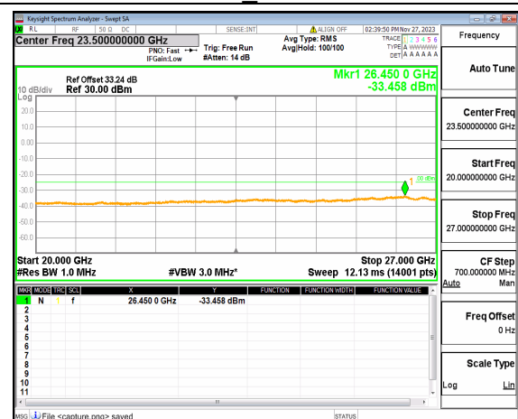
n41 (20GHz-27GHz) 60M DFT-s-OFDM QPSK Edge_1RB_Left Low
