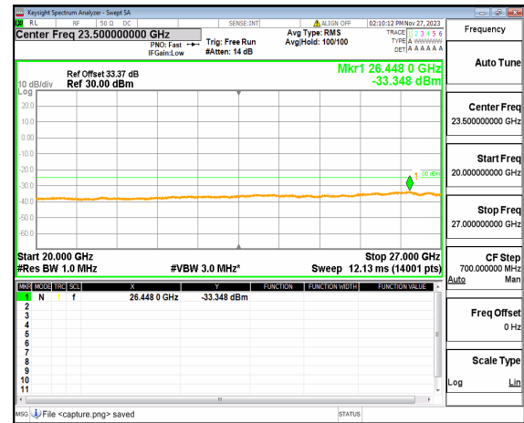
n41 (20GHz-27GHz) 40M DFT-s-OFDM QPSK Outer_Full High
