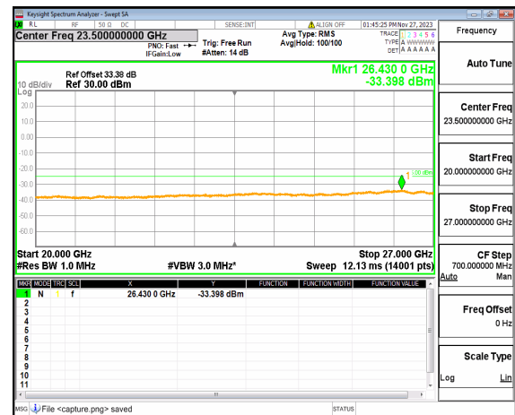
n41 (20GHz-27GHz) 30M DFT-s-OFDM BPSK Outer_Full High
