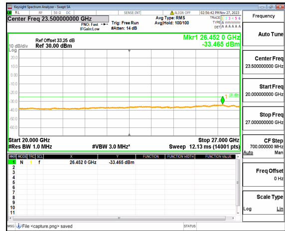
n41 (20GHz-27GHz) 70M DFT-s-OFDM BPSK Outer_Full Low
