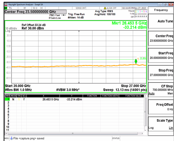
n41 (20GHz-27GHz) 50M DFT-s-OFDM BPSK Edge_1RB_Right Low
