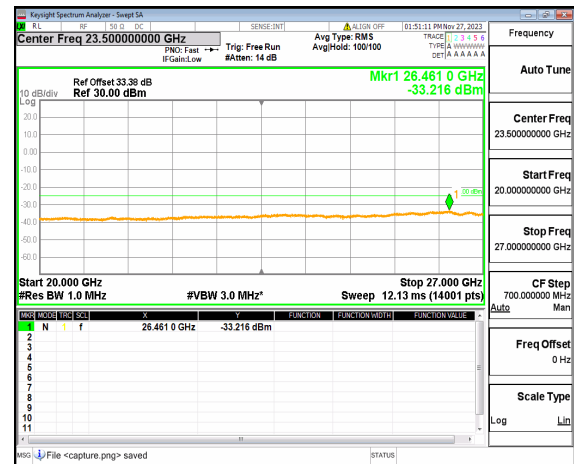
n41 (20GHz-27GHz) 30M DFT-s-OFDM QPSK Edge_1RB_Right_High
