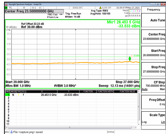
n41 (20GHz-27GHz) 40M DFT-s-OFDM BPSK Edge_1RB_Right Low
