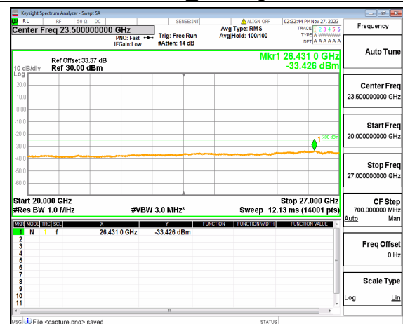
n41 (20GHz-27GHz) 50M DFT-s-OFDM QPSK Edge_1RB_Left High
