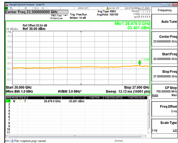
n41 (20GHz-27GHz) 60M DFT-s-OFDM BPSK Edge_1RB_Right Low
