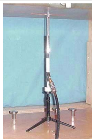
835MHz Dipole Setup
