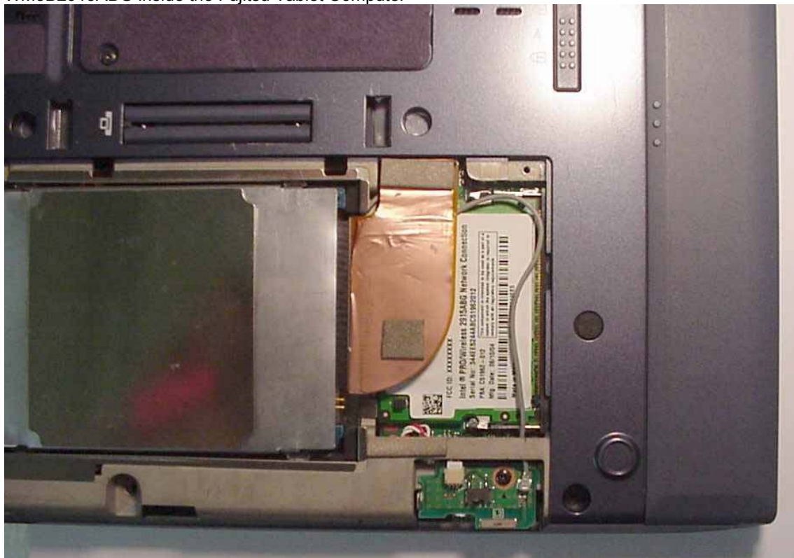
WM3B2915ABG inside the Fujitsu Tablet Computer
