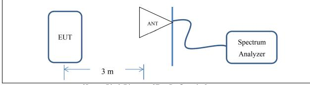
[System Block Diagram of Test Configuration]
