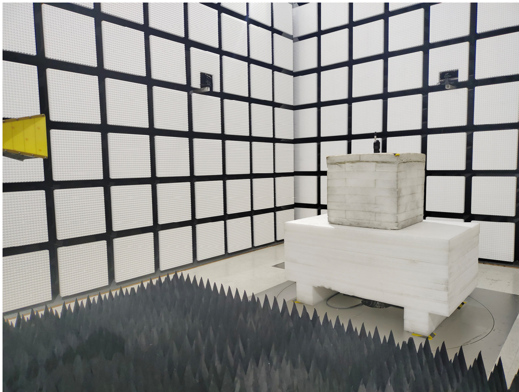
Radiated Emission Above 1GHz View
