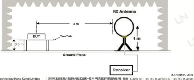
adiated Emission Test-Up Frequency 30MHz~1GHz
