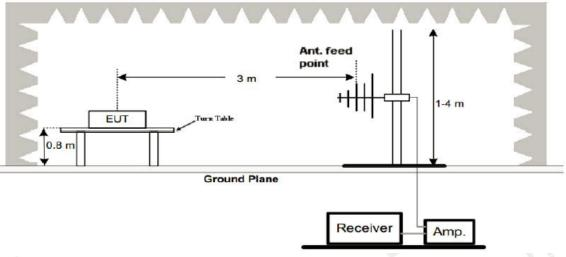
3. Radiated Emission Test-Up Frequency Above 1GHz
