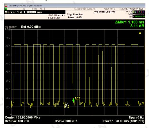
The graph shows the duration of 'on' signal. From marker 1 to marker 2, duration is 560 µs.
