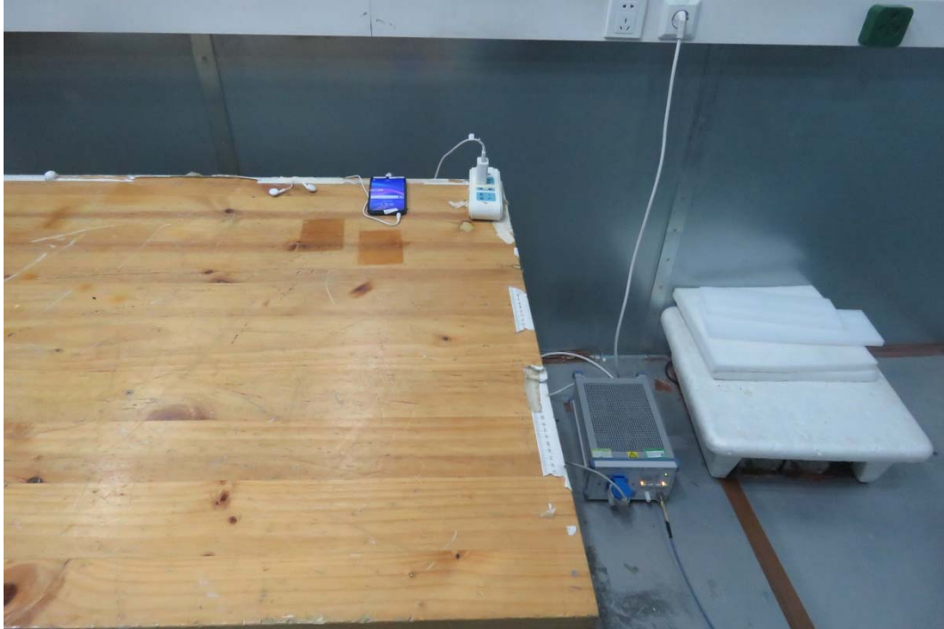
Picture 2 Conducted Emission Test Setup
