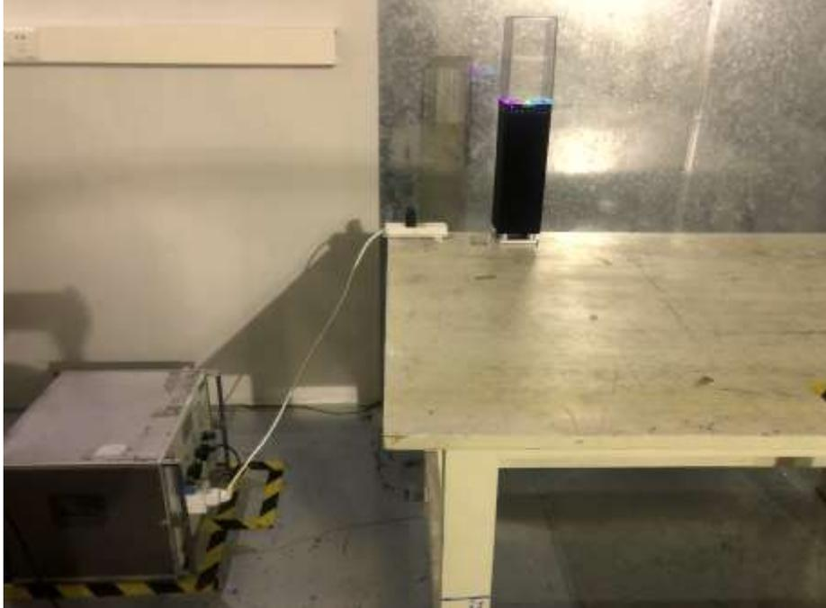
Transmitter Radiation Measurement below 1GHz
