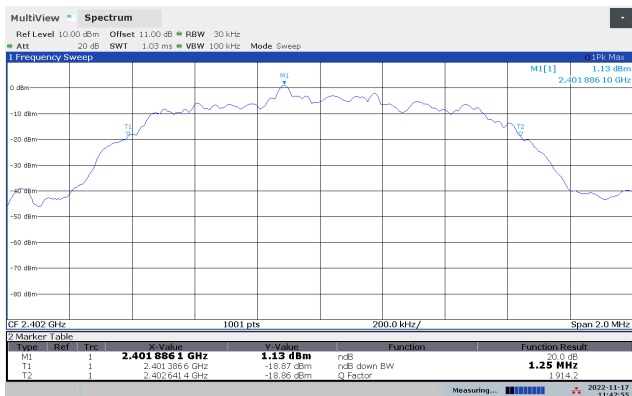
20dB Bandwidth 2402 MHz, 8-DPSK
