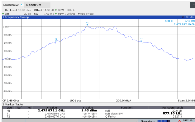
20dB Bandwidth 2480 MHz, GFSK
