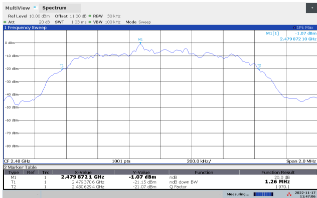
20dB Bandwidth 2480 MHz, 8-DPSK
