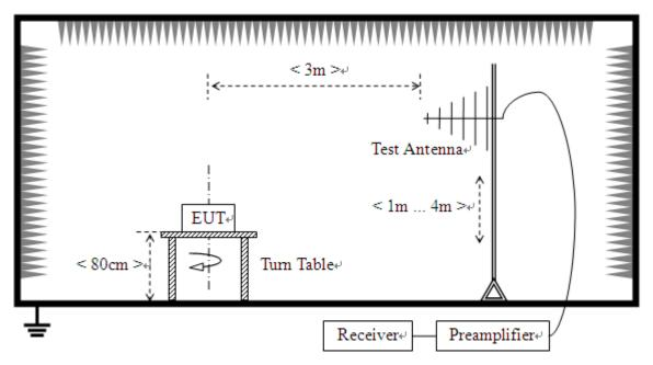
(For the test frequency from 30MHz to1GHz)
