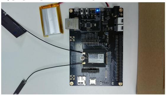
The Particle B402 is a mesh and Bluetooth development kit designed for building connected projects and products. To set up the device you'll need an Android or iOS mobile phone and a connection to the internet.
