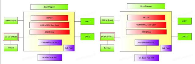
The function of both 8077 and 8088 in the circuit is to convert a 5V voltage to a 3.3V voltage. The only difference between the 8077 and 8088 is that the input voltage range is not the same.
