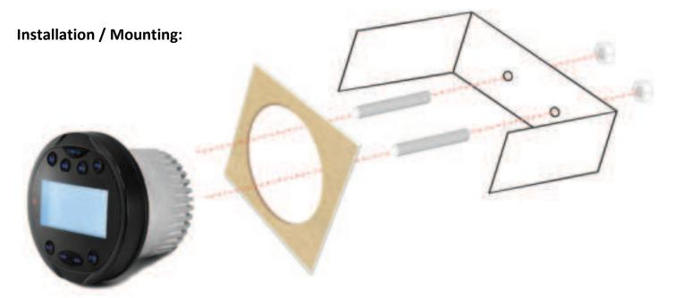
Be sure to install the U-shaped bracket so it fits flush to the interior of the mounting wall. The receiver face should sit flush on your dash / console panel.
