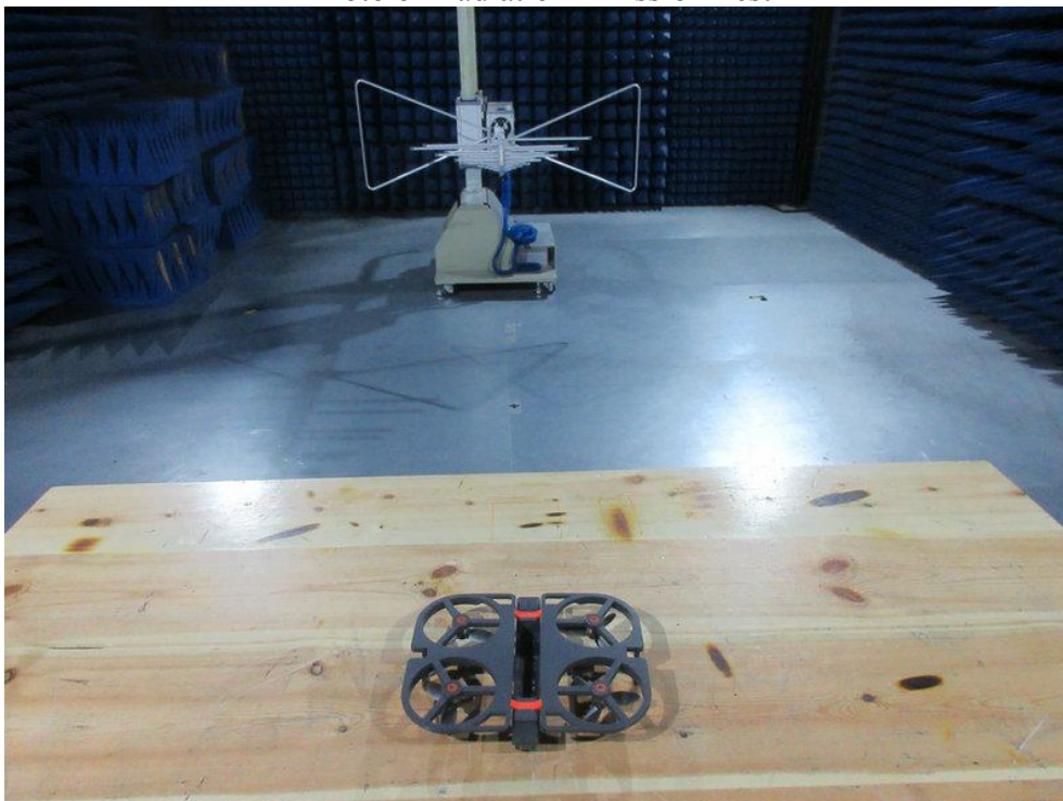
Photo of Radiation Emission Test
