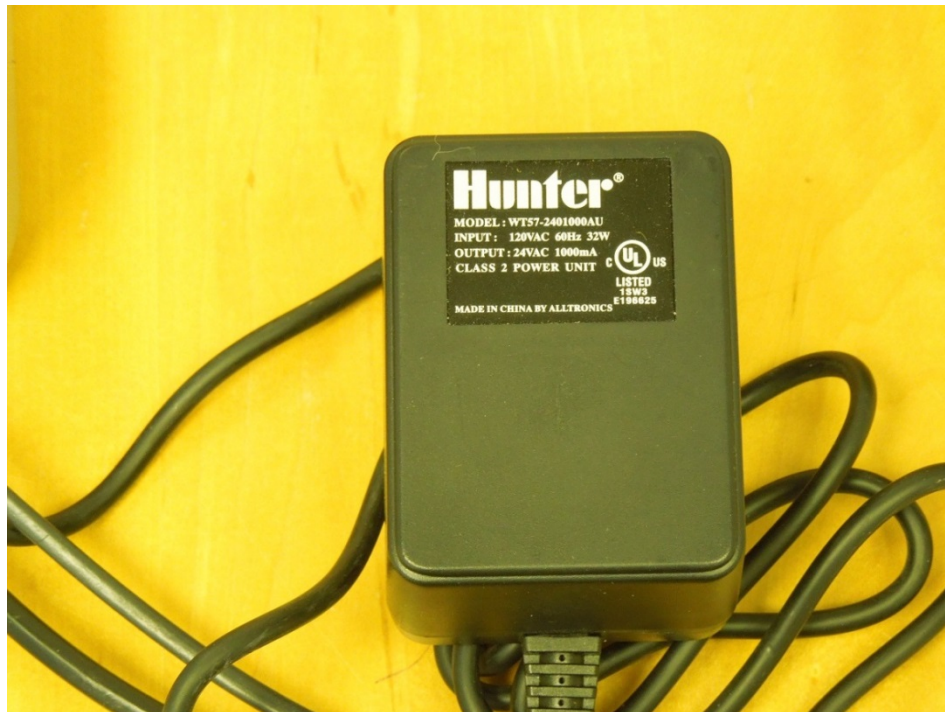
Irrigation Controller 24 VAC transformer (not made by IrriGreen)
