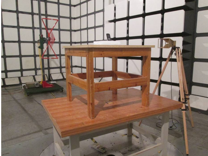
Radiated Emissions Test View (Below 1 GHz)
