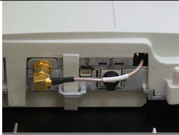
Figure 15 – internal (service) antenna cable, manual power selector, and auxiliary jack on the left side
