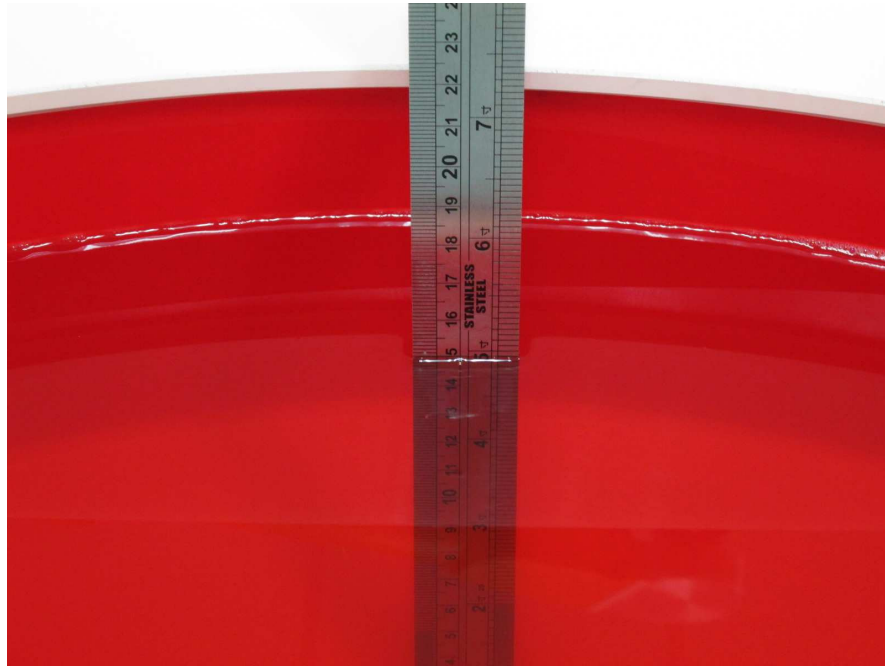
Fig 8.3 Photo of Liquid Height for Body Frequency 2450MHz
