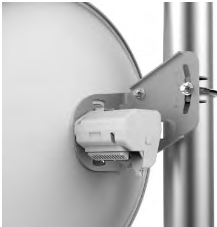
Figure 7 Force 300-25 module mounting bracket
