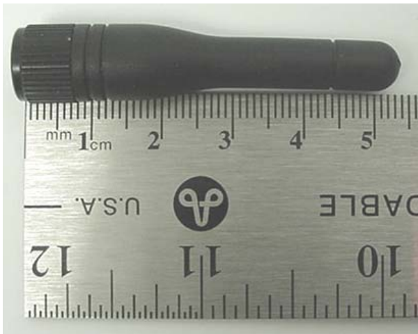
Dual-Band CDMA Antenna - \frac{1}{4} wave Helix
