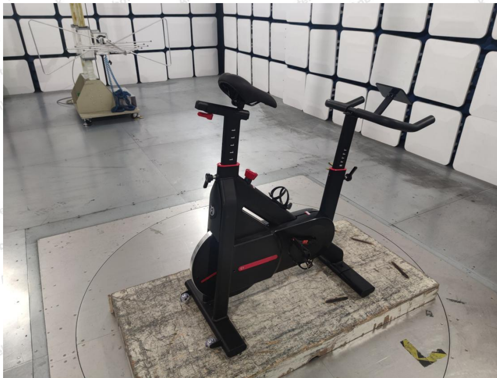
Photo of Radiation Emission Test
