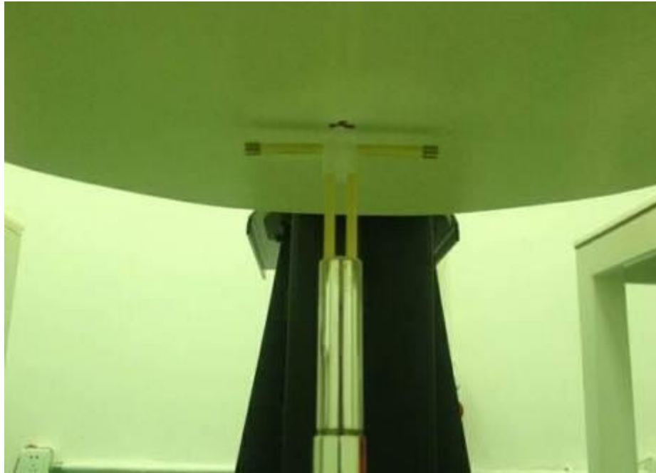
Picture 8.2 Photo of Dipole Setup
