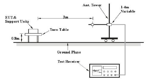
The radiated emissions were performed in the 3 meters distance, using the setup accordance with the ANSI C63.10-2013. The specification used was the FCC 15.209 and FCC Part 15.237(b) & 15.237 (c) limits.
