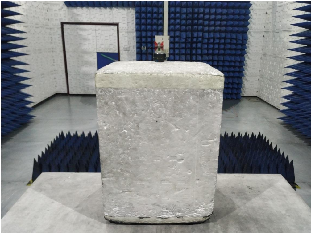
RADIATED EMISSION TEST SETUP ABOVE 1GHz
