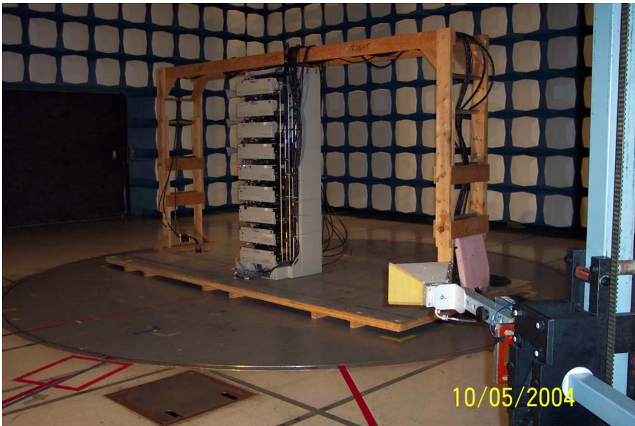
Figure 16 RE 1 GHz – 10 GHz EUT Configuration
