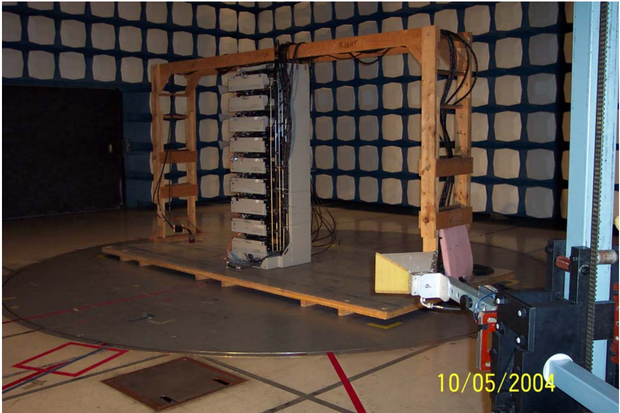
Figure 5 RE 1 GHz – 18 GHz EUT Configuration
