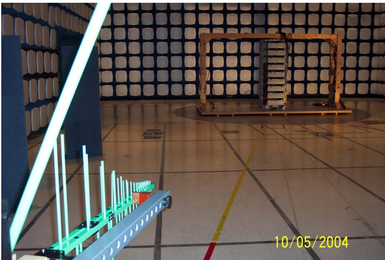
Figure 4 RE 30 MHz - 1 GHz EUT Configuration
