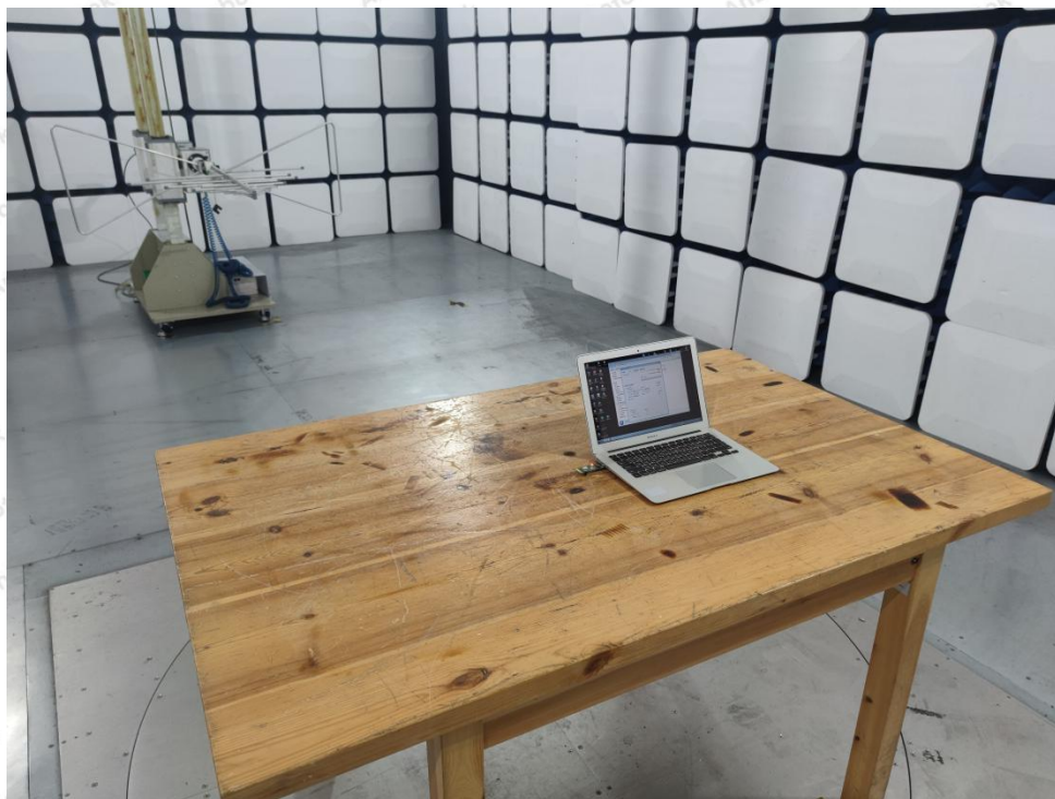
Photo of Radiation Emission Test
