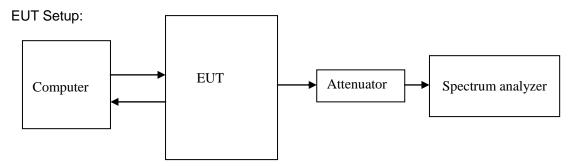
REMARKS: Attenuator loss (dB)=40dB, Cable Loss (dB)=1.5dB.
