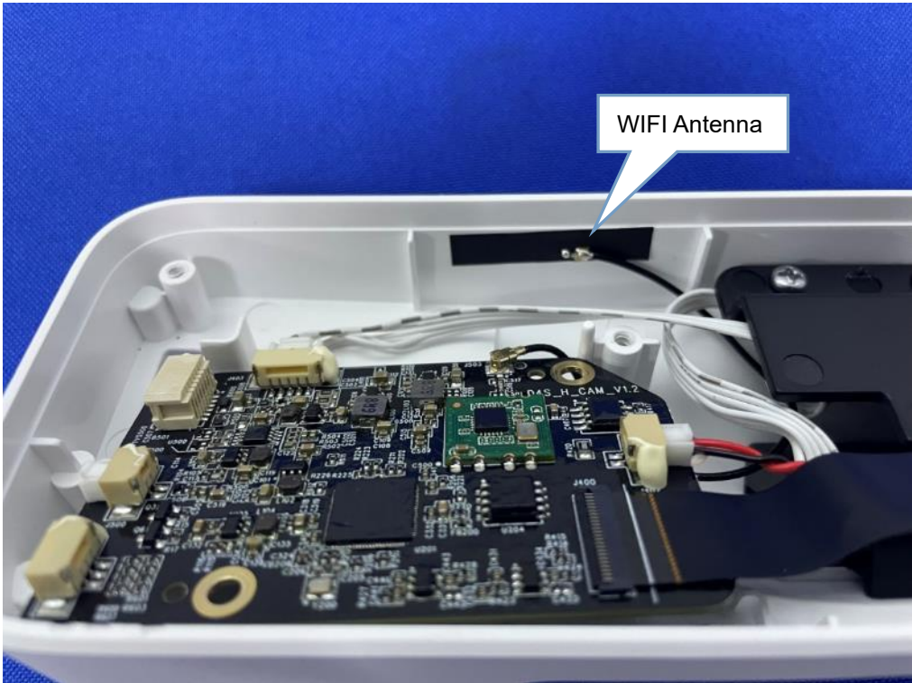
WIFI Antenna position
